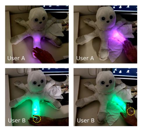
Fig. 2. In this functional test, the toy responds with magenta color to user A and with green to user B. The discernment is possible thanks to the small, discreet magnetic ring worn by user B (highlighted in yellow) which is detected by the sensors. The shown prototype, as a work-in-progress, is still partially disassembled: all electronics will be hidden by an external envelope. (Color figure online)
