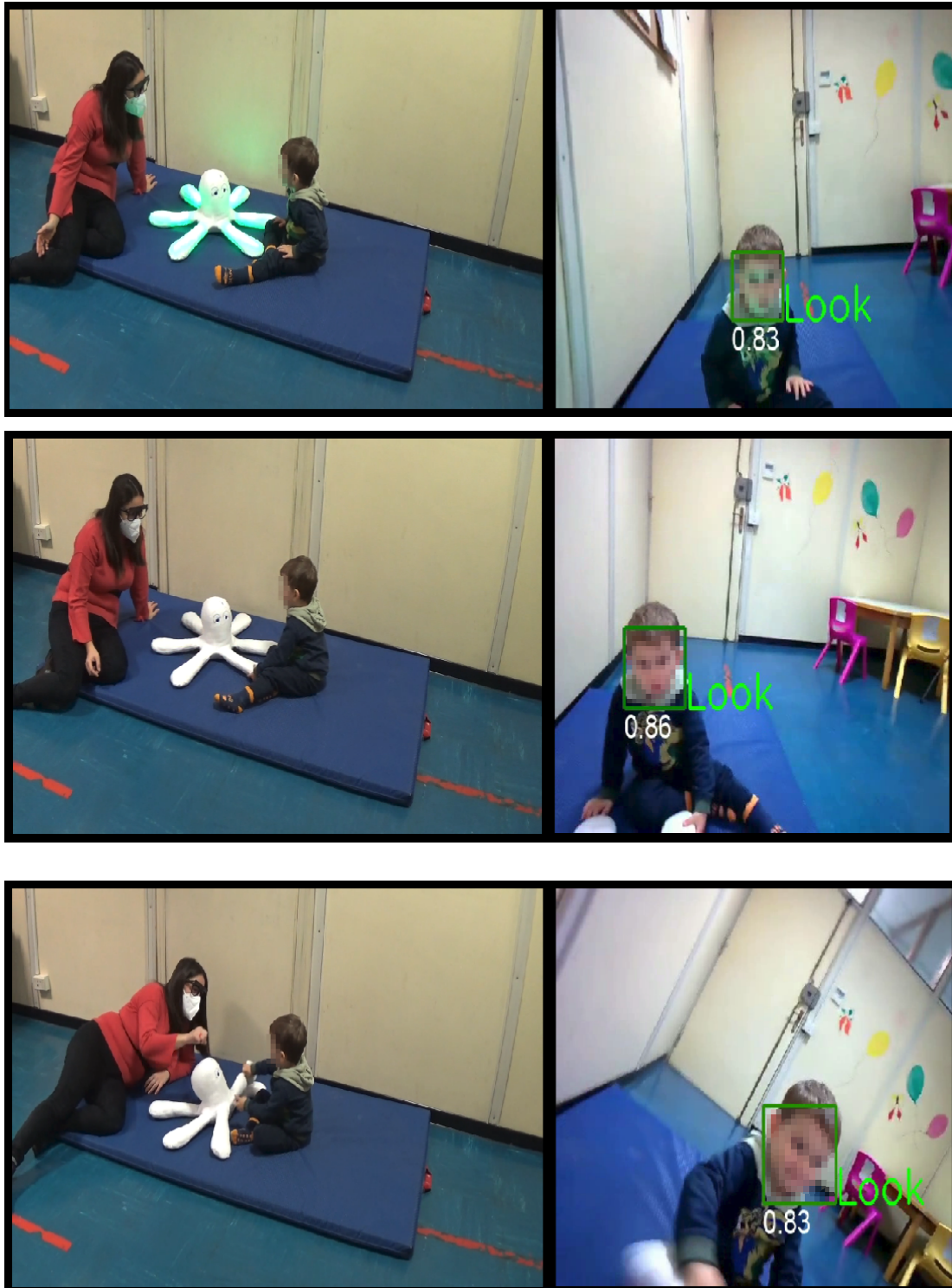
Figure 21: 3 images showing how the gaze detection system properly detects the eye contact between the child and therapist, who wears the sensorised glasses (on left the environmental camera images, on right the glasses camera images).
