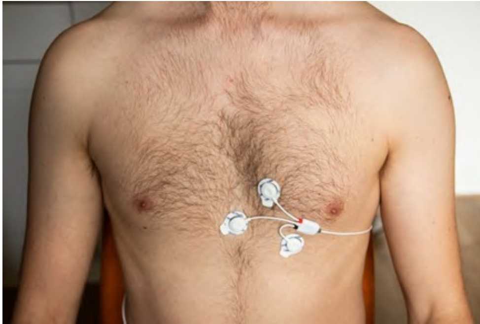
Figure 4: Wet electrode setup. Gelled electrodes were attached to the skin using an adhesive membrane to function as a baseline for the dry electrode setup. Electrodes were configured in the same V2 configuration as the dry electrodes.
