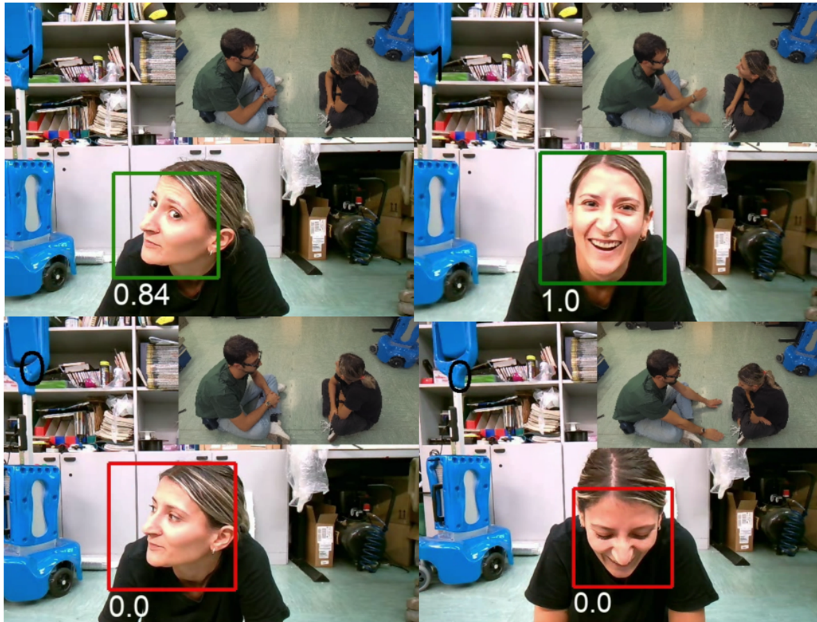
Figure 20: a test run in the lab, to assess the accuracy of the eye contact detection.
