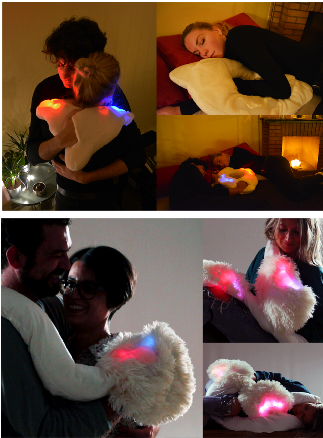
Figure 2: Evolution of Lokahi design. Top: the first version of the device Lokahi . Bottom: the current design improves the usability of the device as the new shape allows users to place Lokahi freely on the body, to observe the visual feedback easily.
