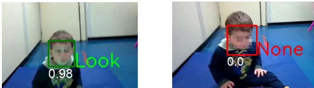
Figure 6. An example of output by camera glasses during a test with a child. Left: when the child looks at the therapist, the output of Artificial Intelligence indicates this event with a green box and the probability that the child is actually looking into the eyes is shown. Right: the AI output produces a red box when no eye contact is detected.
