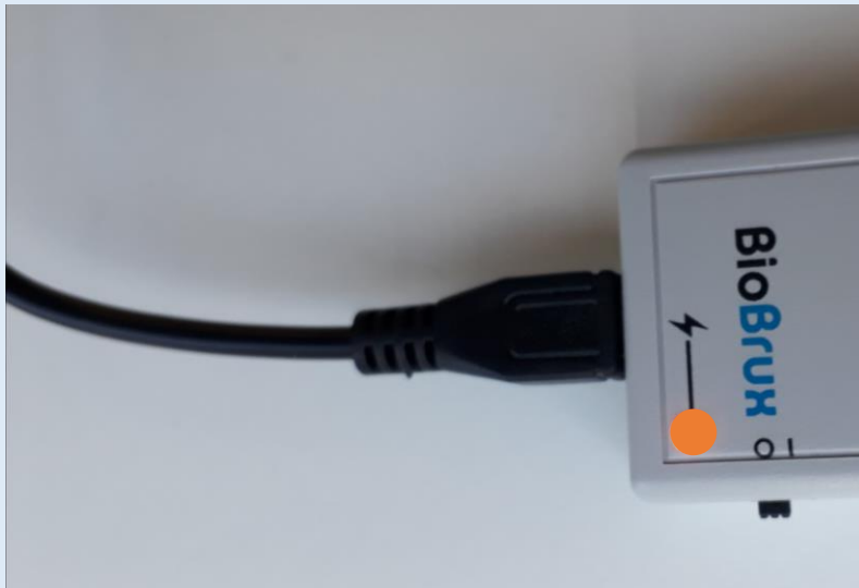
Figure 21 Device charging, LED orange.
