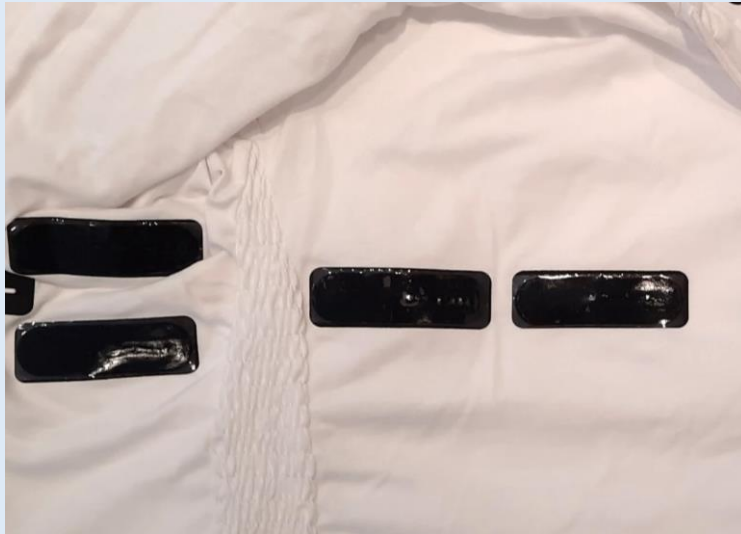
Figure 13 T-shirt electrodes with plastic protection foil, inner layer.
