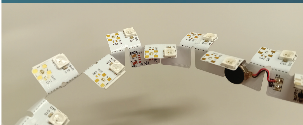
Fig.10: Flexible electronics embedding sensors (touch and IMU sensors) and actuators (RGB LEDs strips, vibrating mini discs, speakers), placed in Panda PlusMe paws. The design (under patenting) allows to withstand the mechanical stress in the 3 axes.
