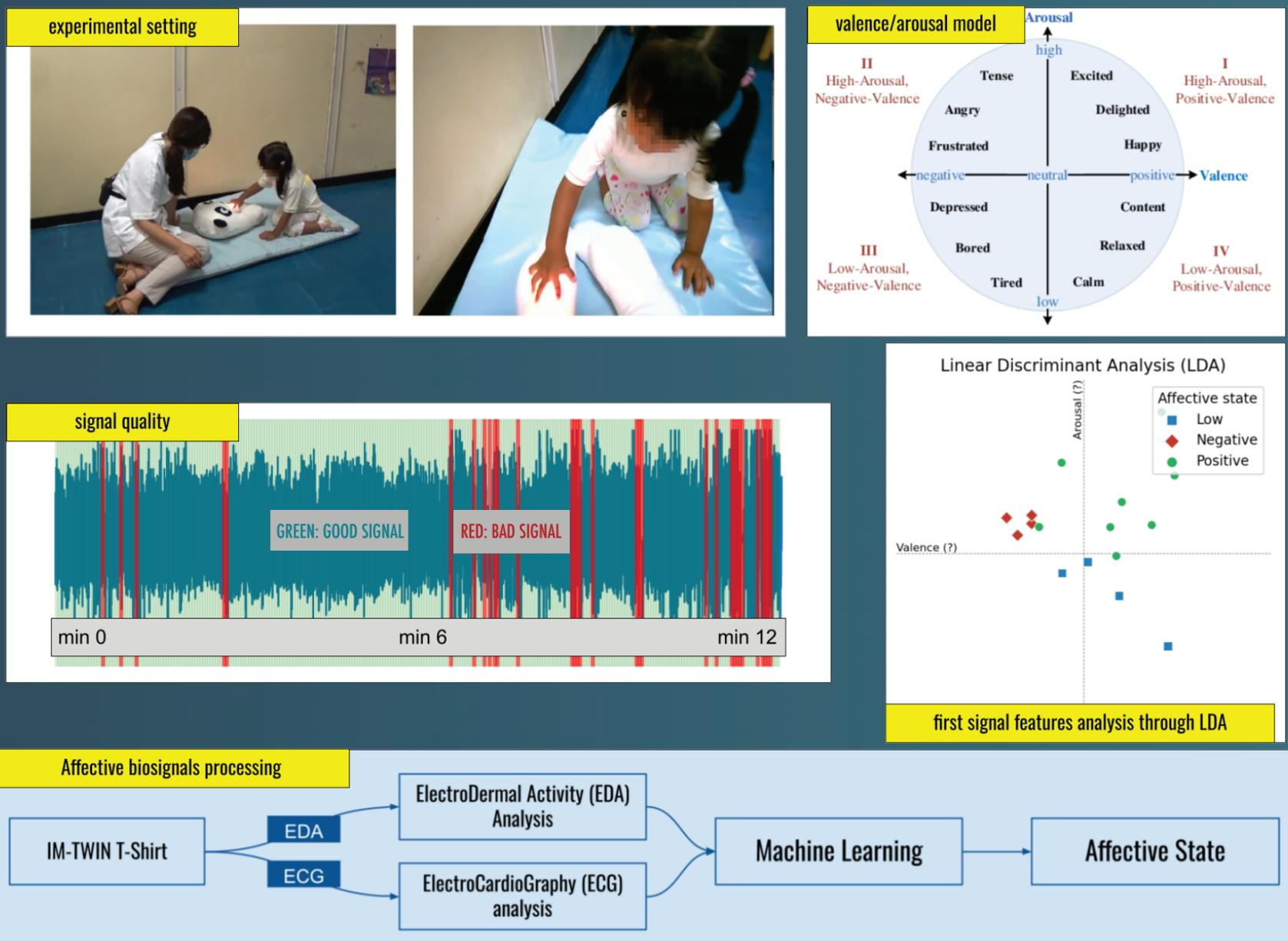
Fig. 16: a 12 minute long test, where an ASD child is involved in a play activity with the therapist and PlusMe. The initial analysis shows how the t-shirt signal is usable (about 90% of data features a good quality), and can potentially be used to categorise the child's effective states (low, negative, positive engagement state) through machine learning algorithms.
