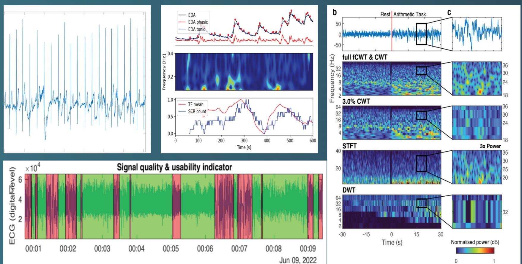
Fig. 17: the EDA and ECG signals collected by the t-shirt are pre processed through the fCWT, a novel fast and accurate time frequency method, developed in the project, to reliably cope with the noise which characterises the physiological data.
