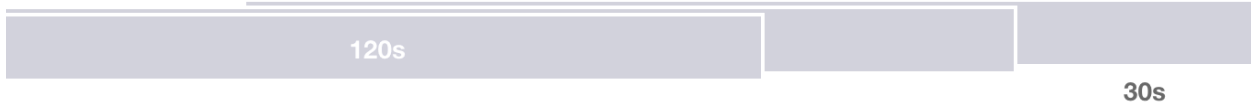
Figure 7: ECG is analyzed using a 30s window and a 120-second trailing window having a stride length of 30 seconds for time and frequency-based HRV metrics, respectively. The window trails analysis instead of surrounding the analysis. The latter would require looking into the future which would impair real-time analysis.
